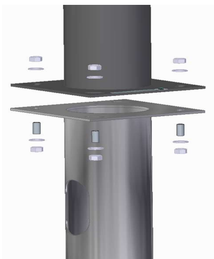
Place tubes, screws M14, washers and nuts M14
