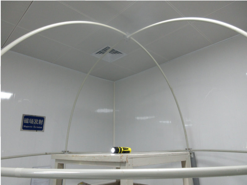
Photo of Magnetic Radiated Emission Test
