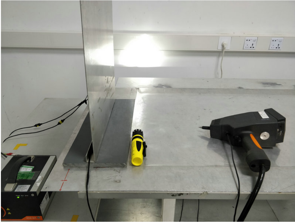
Photo of Electrostatic Discharge Immunity Test
