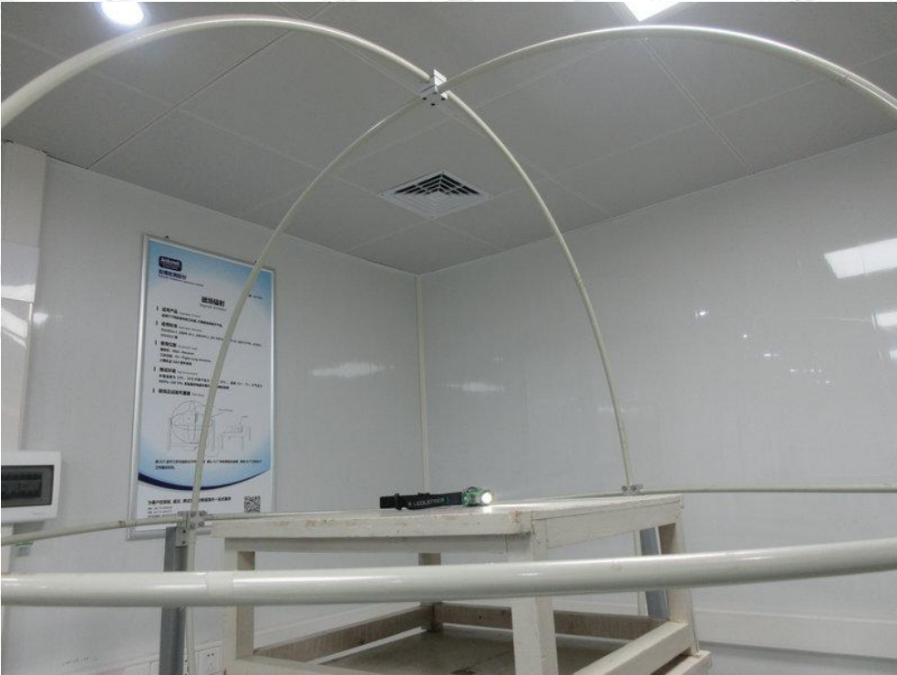
Photo of Magnetic Radiated Emission Test
