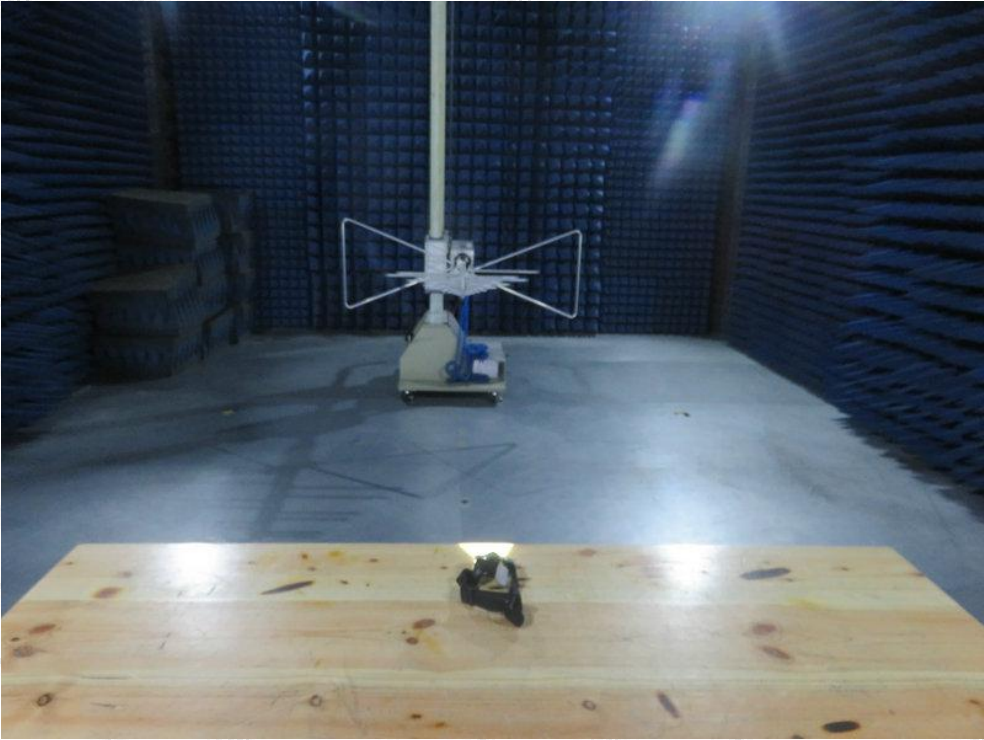
Photo of Radiated Emission Test
