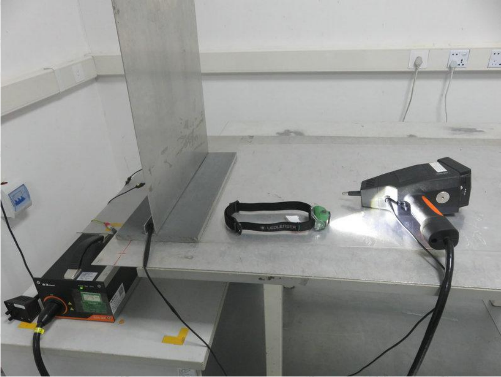
Photo of Electrostatic Discharge Immunity Test
