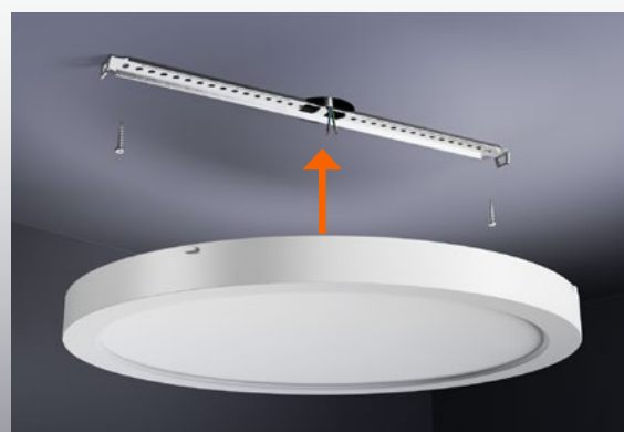
SURFACE-MOUNTED INSTALLATION For ceilings without cut-outs: remove springs and mount rail directly. For On/Off and sensor versions only.
