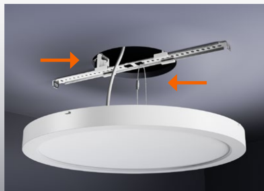
Attach the luminaire using the safety wire, connect it to the power supply and snap it into the rail.
