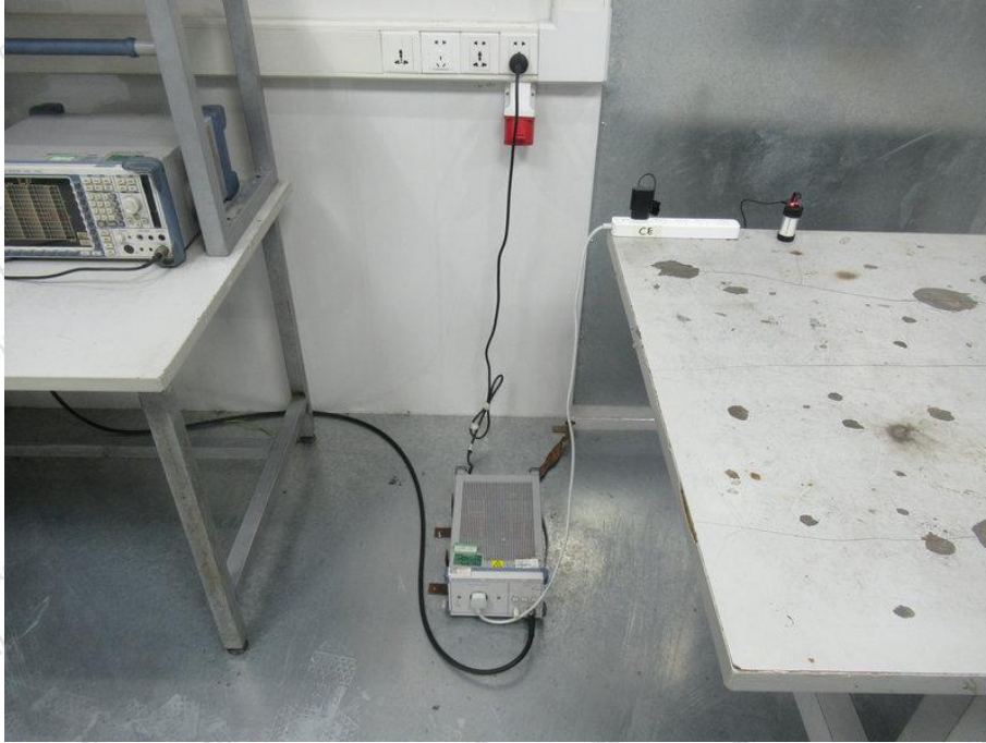
Photo of Power Line Conducted Emission Test
