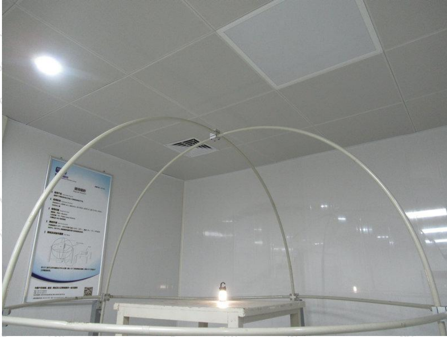
Photo of Magnetic Radiated Emission Test
