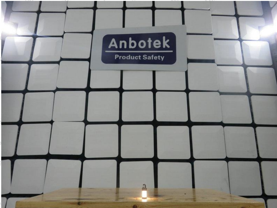
Photo of RF Field Strength susceptibility Test
