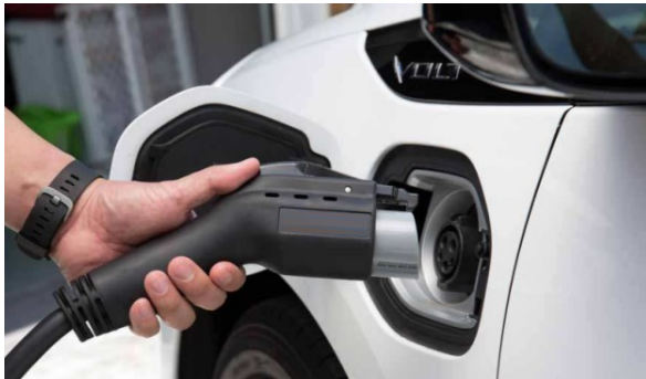
Step 1: Plug in the charging gun
